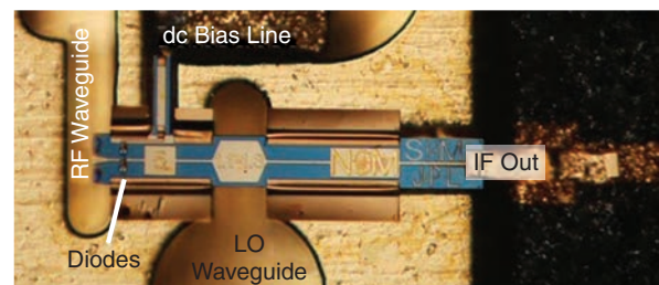
Figure 6. A 1.2-THz mixer device mounted in its housing. (Source: [28].)
