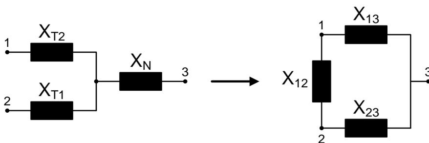
$$X_{12} = \frac{X_{T1} \cdot X_{T2} + X_{T1} \cdot X_{TN} + X_{T2} \cdot X_{TN}}{X_N} = \frac{35675 \text{m}\Omega^2}{55 \text{m}\Omega} = 648,63 \text{m}\Omega$$
