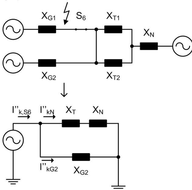
$$X_{\text{ges}} = \frac{(X_T + X_N) \cdot X_{G2}}{X_T + X_N + X_{G2}} = \frac{(70,18 + 55) \cdot 141,67}{70,18 + 55 + 141,67} \text{ m}\Omega = 66,46 \text{ m}\Omega$$
