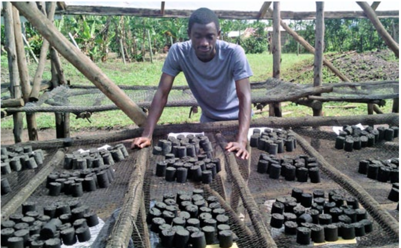
Development of rice and coffee husk briquettes as sustainable fuel sources for domestic cooking applications in Uganda. PHOTO BY MICHAEL LUBWAMA.
