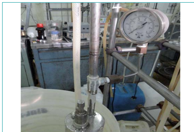
Fig. 1 A view of the experimental setup for testing of the RFD based fluidic pump
