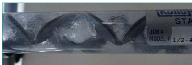
Fig. 1 Static mixer internals
