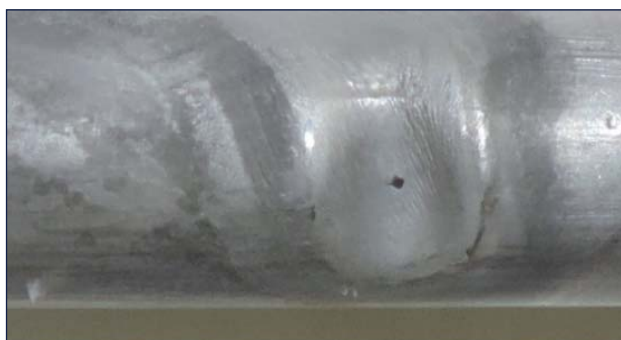
Fig. 2 Punctured target tube after experiment 3
