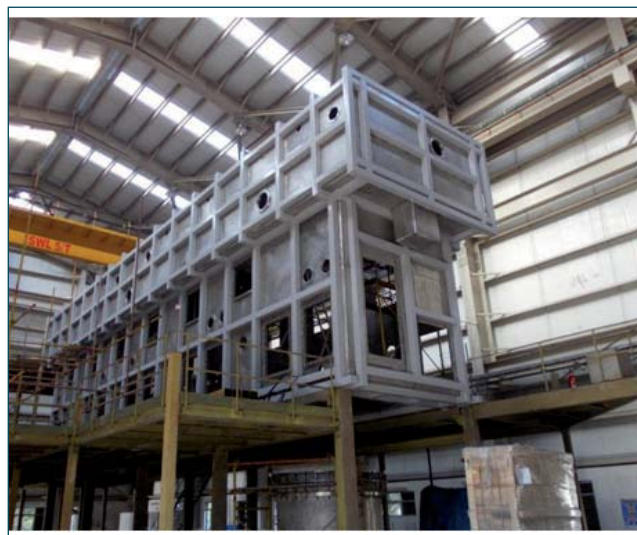
Fig. 1 Erected containment box
