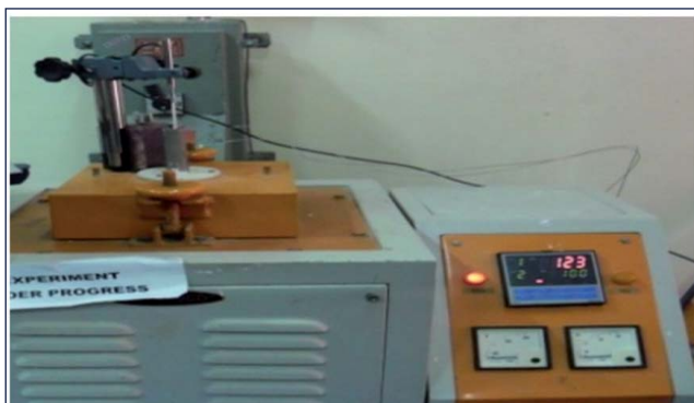
Fig. 2 Out-of-pile experimental set up arrangement with capsule loaded in electric furnace
