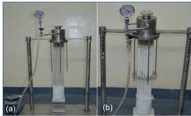
Fig. 1 Experimental set up for Y_2O_3 (a) before and (b) after coating
