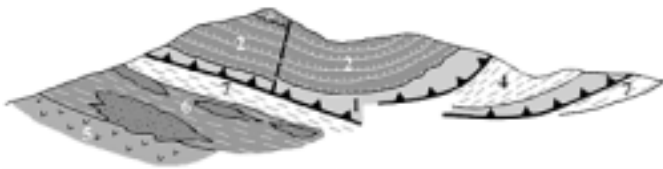
FIGURE 2—Schematic section showing the geometrical relations between the Marecchia sheet Ligurid Complex and the Umbro-Marchean-Romagna Succession. Legend: MARECCHIA SHEET LIGURID COMPLEX – 1. Ligurid Complex; 2. Campaolo Fm.; 3. S. Marino Fm.; 4. Arenarie di Perticara Fm.; UMBRO-MARCHEAN-ROMAGNA SUCCESSION – 5. Marnoso-Arenacea Fm.; 6. “Colombacci” Fm.; 7. Peliti grigio-azzurre Fm. (from Bortolotti et al. , 1992, modified).
