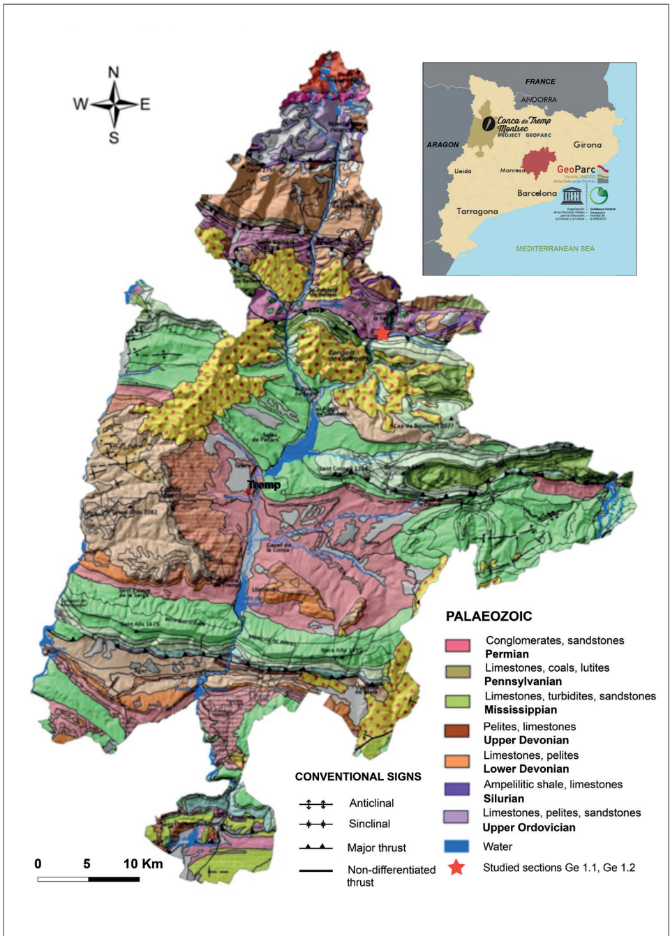
Fig. 1. Geological map of Conca Trep-Montsec Geopark Project with position of sections Ge 1.1 and Ge 1.2.
