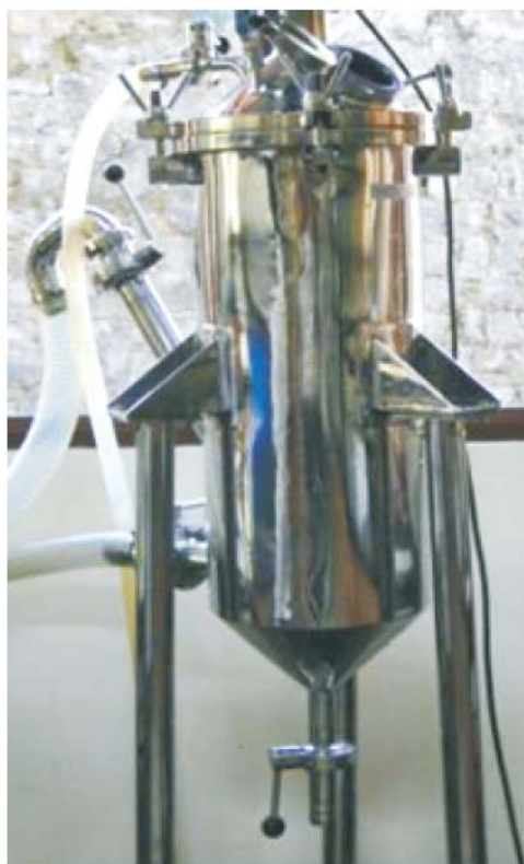
Fig. 67 Prototype for seed separation from apple pomace: Conceived and designed at CSIR-IHBT
