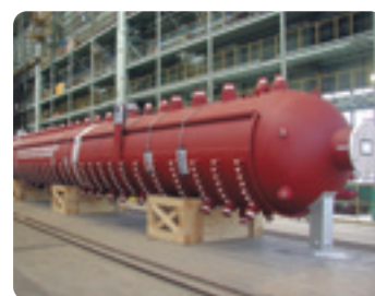
Steam drum for the Tanjung Bin Power Project in Malaysia
