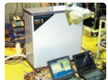
Polymer Electrolyte Fuel Cell (PEFC) system
