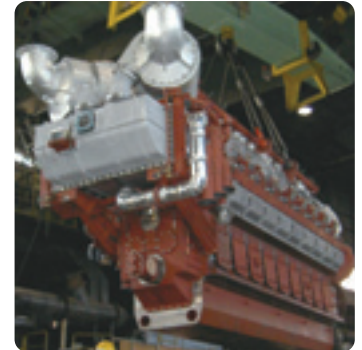
Large-sized gas engine Engine type: Niigata18V28AG Output: 5,500/5,800 kW Speed: 720/750 min -1
