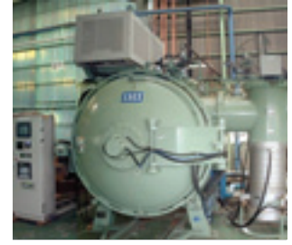
Vacuum heat treatment furnaces
