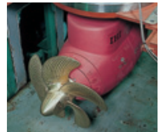
Superconducting motor installed in a ship propulsion unit
