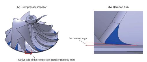
Fig. 5 Ramped hub
