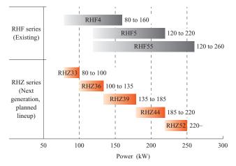
Fig. 2 Comparison of lineups between RHF series and RHZ series
