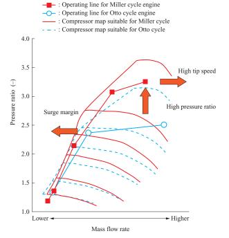
Fig. 1 Engine operating line and compressor map
