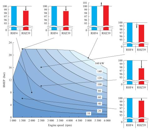
(Note) The vertical axis of the bar graphs indicates the specific fuel consumption (%).
