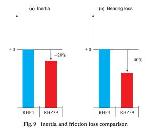
achieving a good balance between mechanical loss and rotational stability.
