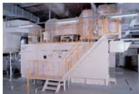
2,000-kW-class IM270 gas turbine
