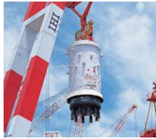
Reactor pressure vessels
