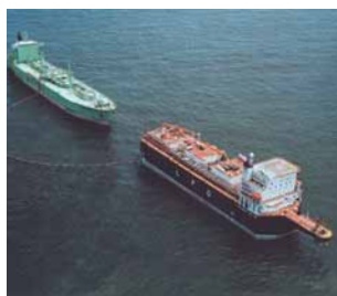
LPG floating storage offloading units
