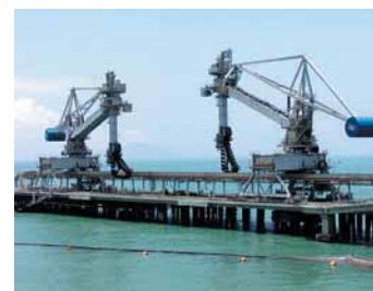
Continuous ship unloaders like the one delivered to East Asia
