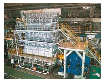
Electronic-controlled large, low-speed marine diesel engine
