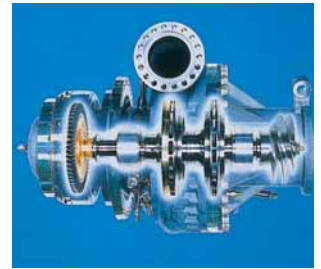
Liquid hydrogen turbopumps
