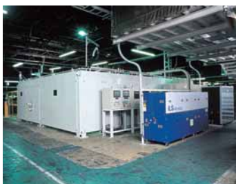
Outside view of the tailored-blank welding system using LD-pumped YAG laser
