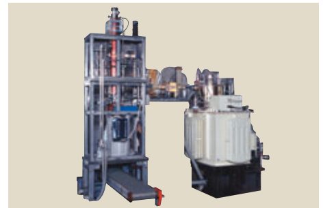
10-MeV 1.5-kW electron-beam accelerator device
