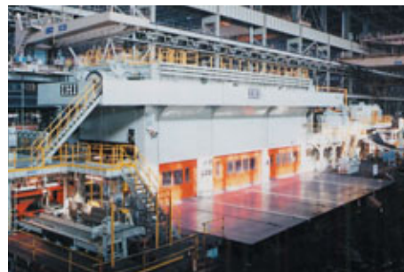
This 5,850-metric ton transfer press has already been delivered to GM in the United States.
