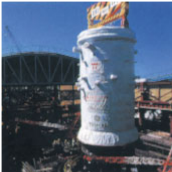
Reactor pressure vessels
