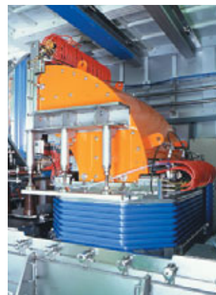
Device exterior of large-scale ion implanter with mass separator
