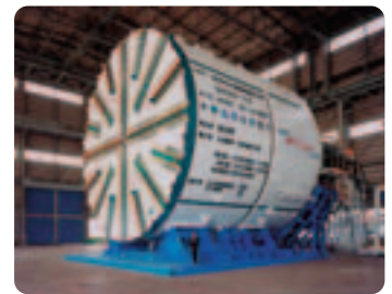
Completed large-scale shield tunneling machine for the Akita Chuo Expressway project
