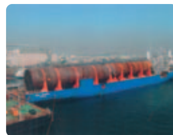
Shipment of large GTL reactor
