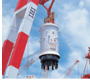
Reactor pressure vessels
