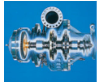
LE-7A liquid hydrogen turbopumps
