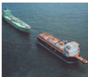
LPG floating storage offloading units
