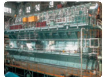
Electronically controlled 12RT-flex96C common-rail marine diesel engine
