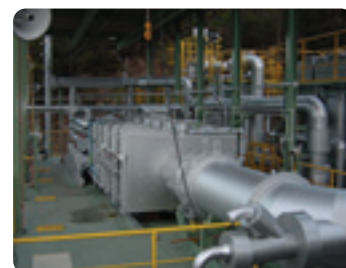
Coal combustion test furnace (coal combustion capacity of 150kg/h)
