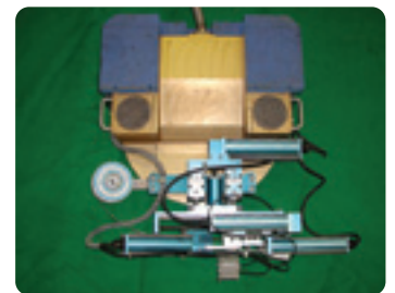
Underwater laser repair welding machine
