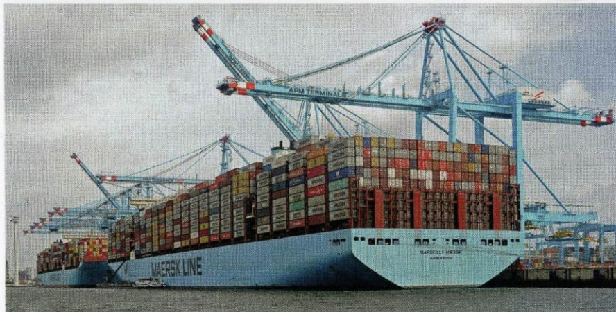
Maersk Line container ships: Typical loads are a mix of 20-foot and 40-foot (2-TEU) ISO-standard containers, with the latter predominant.
