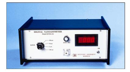
Digital Nanoammeter, DNM-121, a rugged and low cost instrument, is a product of extensive R&D using high input impedance integrated circuits. It has 4 decade ranges with 100% over-ranging. The unit is suitable for current measurement in the range of 100pA to 200 $\mu$ A. For the ease, readings are directly obtained on a 3½ digit DPM. The instrument is capable of accepting either polarity of the input current.
