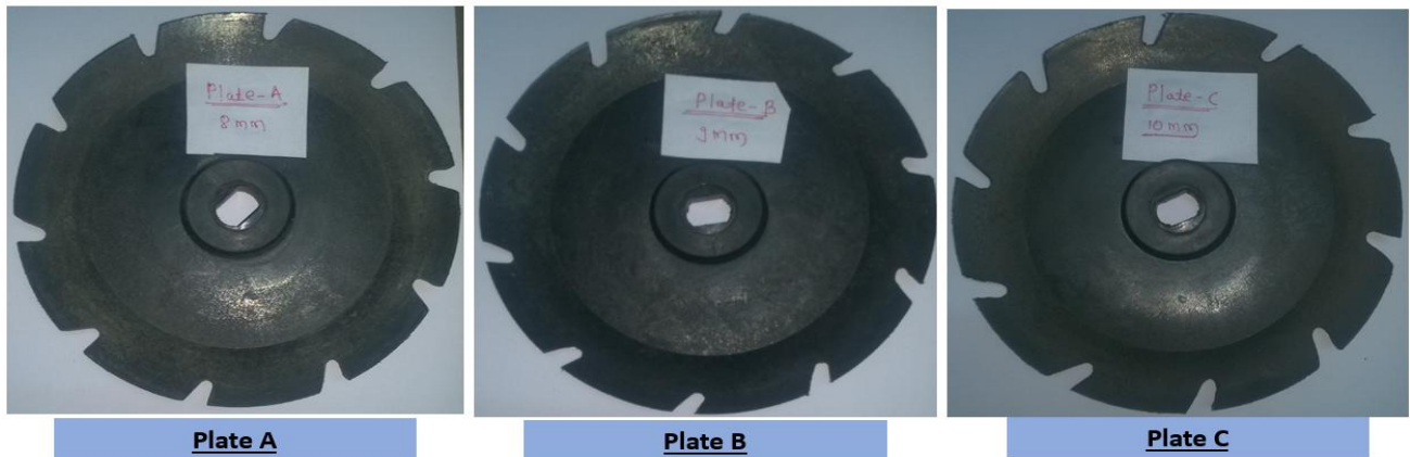
Fig.3 Metering plates used for metering of soaked okra seeds
