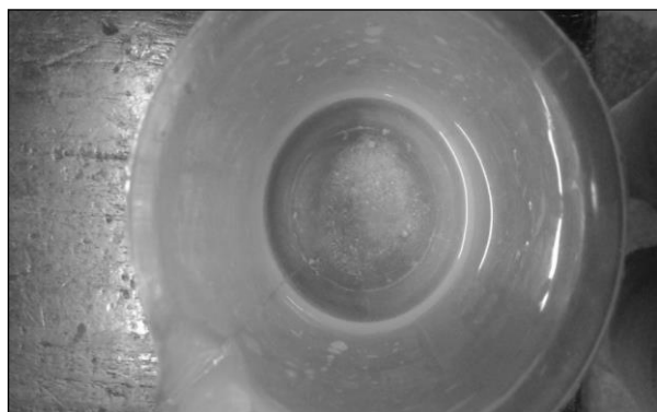
Fig. 1. Unmixed NaCl crystal in the solution beyond saturation limit
