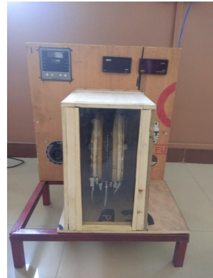
Fig. 1. Setup of Thermal Composite of Composite Wall
