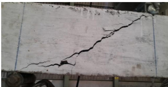
Figure 9: Failure pattern of L.B.1x6 beam
