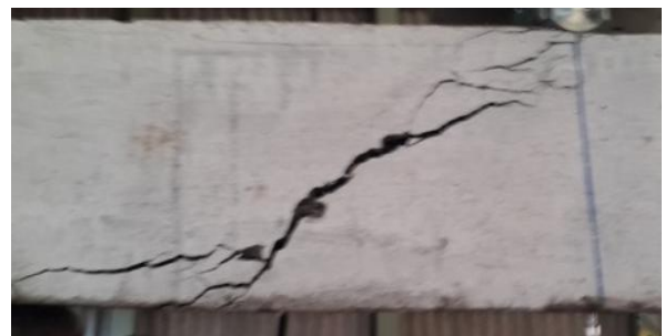
Figure 11: Failure pattern of L.B.1x8 beam
