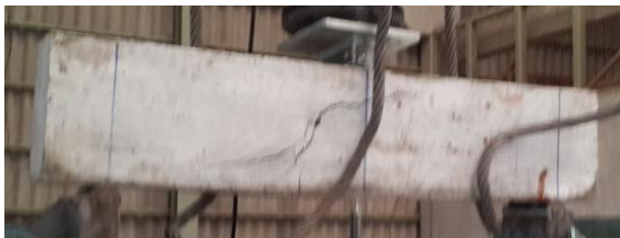
Figure 15: Failure pattern of L.B.2x13 beam
