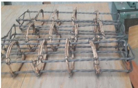
Figure 1: Fixed L.buchananii s shear reinforcements
