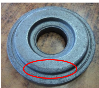
Photograph 2: Unfilling defect at back side of job
