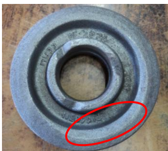
Photograph 1: Unfilling defect at front side of job
