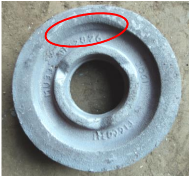
Photograph 1: Unfilling defect at front side of job
