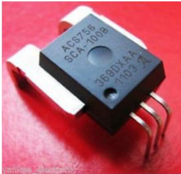
Figure 2. (a)ACS756 sensor (b) General block diagram of ACS 756 sensor
