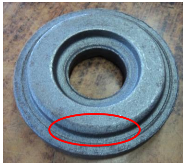
Photograph 2: Unfilling defect at back side of job
