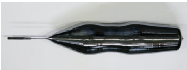
Fig. 4: Test-shape of Si crystal for project "Kilogram-2" grown using the model-based diameter control system developed in IKZ.
