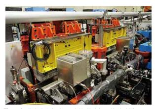
**Figure 2.** Twin Polarization-variable Undulators/Optical Klystron at UVSOR-III.
