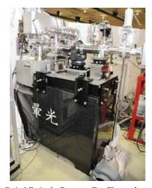
Figure 3. Optical Cavity for Resonator Free Electron Laser.
