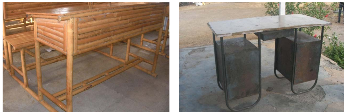
Figure 3. Comparison between two-year-old conventional steel and bamboo furniture
