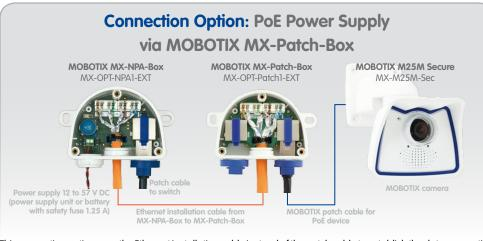
This connection option uses the Ethernet installation cable instead of the patch cable to establish the data connection and PoE power supply. This is helpful, if e.g. an IP camera on a high pole is connected to the network installation cable via the MOBOTIX MX-Patch-Box and the power and network connections are to be supplied through the installation cable at the bottom of the pole using the MX-NPA-Box.
