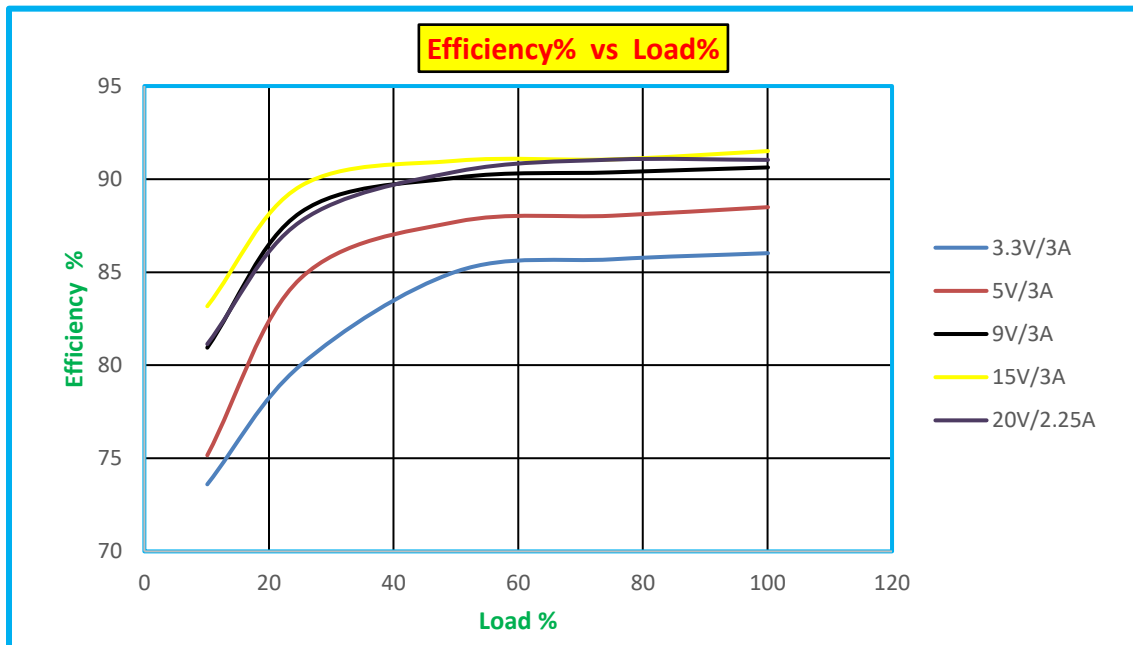
Figure 3-1-2. Efficiency* at 230Vac 50Hz
