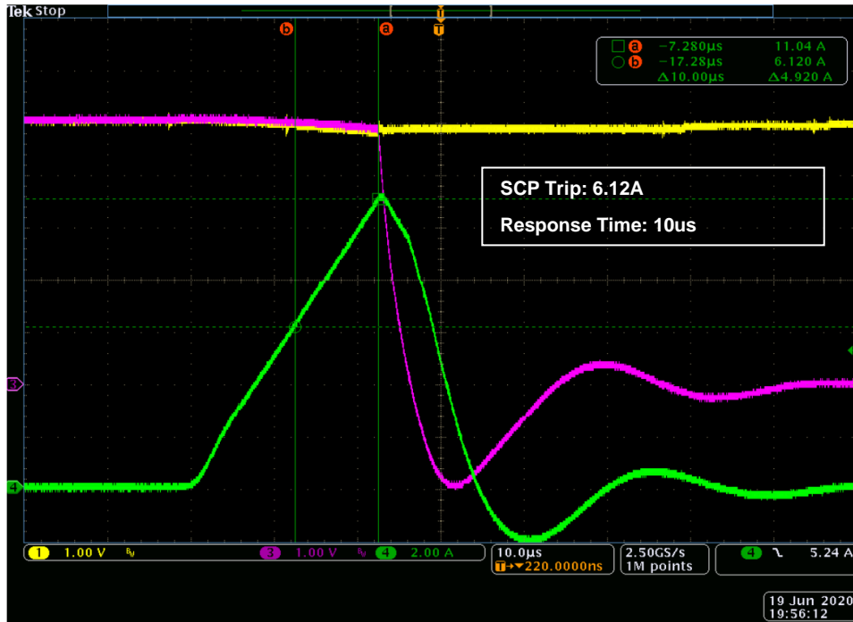
Figure 3-15-1. SCP at 115V, 60Hz (CH3: Vbus_c; CH1: Vbus_in; CH4: Iout)
