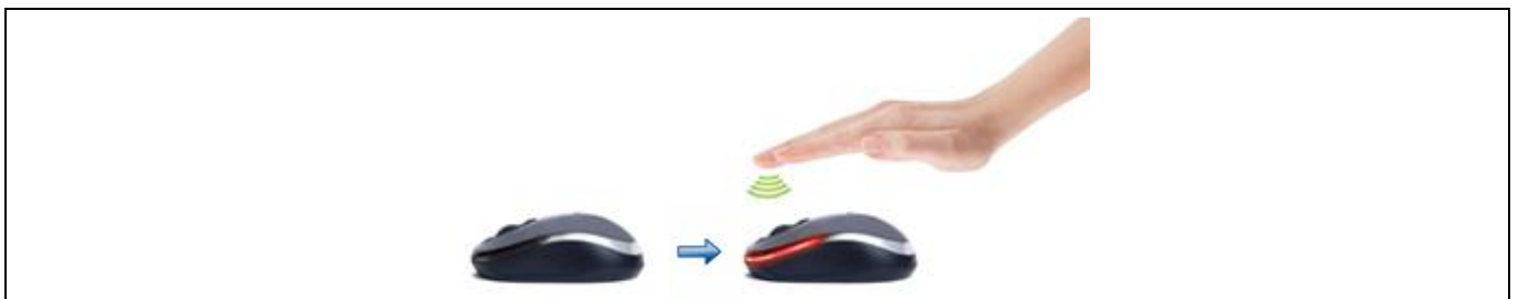
Figure 44 Wake-on-approach implemented in a mouse
