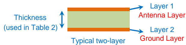
Figure 11. Clarification of PCB Thickness
