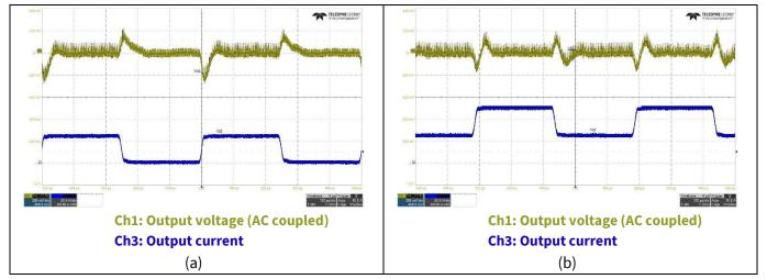
Figure 30 Load-transient response at V<sub>IN</sub> = 48 V - a) load step: 5 percent ↔ 50 percent, b) load step: 50 percent ↔ 100 percent
