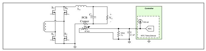
Figure 43 NTC temperature sensing circuit
