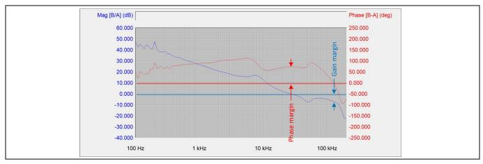
Experimental bode plot (phase margin = 75°, gain margin = 9 dB, crossover frequency = 28 Figure 29 kHz)
