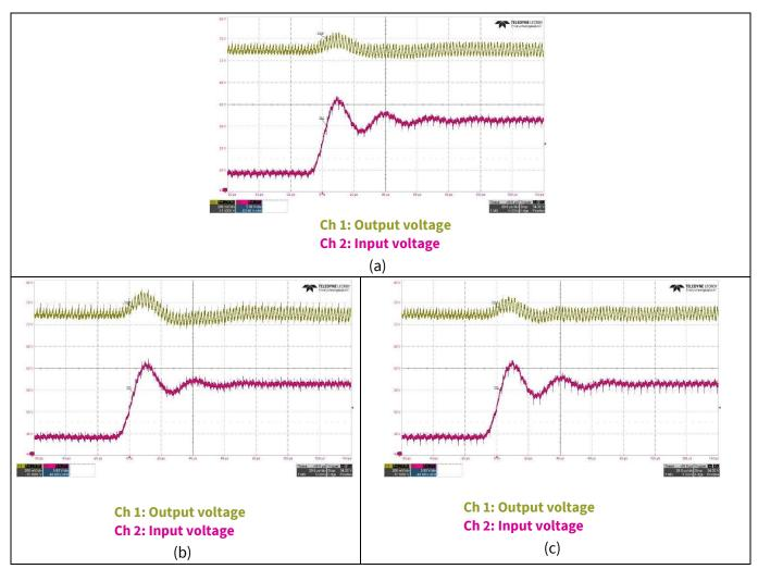
Figure 53 Flux balancing line transient results - a) ramp0\_dutyc\_lock = unchecked (flux balancing disabled), b) ramp0\_dutyc\_lock = checked and fbal\_time\_only = enable (flux balancing is disabled due to DCM), c) ramp0\_dutyc\_lock = checked and fbal\_time\_only = disable (flux balancing enabled with volt × seconds technique)
