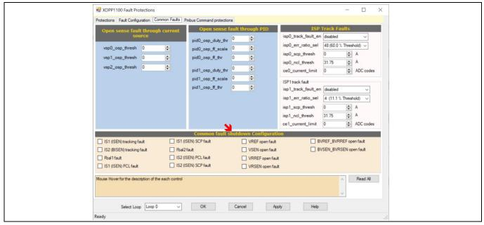
Figure 36 Common Faults tab
