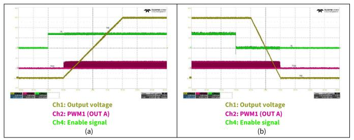
Figure 26 Evaluation kit turn-on and -off delays waveforms at 20 A load - a) TON\_DELAY = 5 ms, b) TOFF\_DELAY = 5 ms
