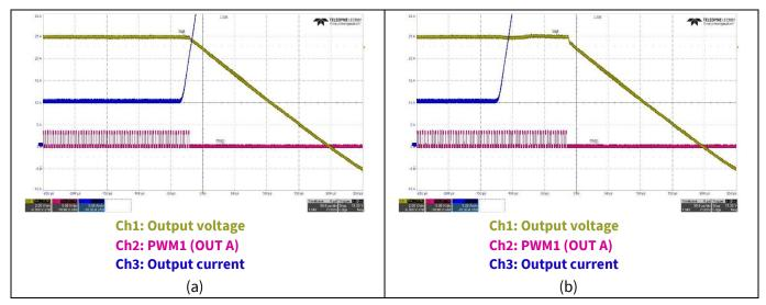
Figure 37 Responses to SCP and OCP (at 48 V input, 12 V output)- a) shutdown by SCP, which responded in one switching cycle, b) shutdown by MFR\_IOUT\_OC\_FAST, which responded after 10 switching cycles
