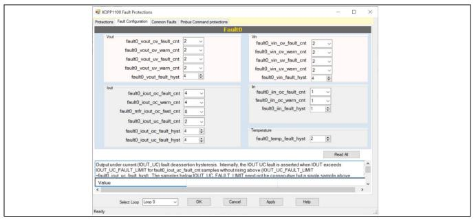
Figure 35 Fault Configuration tab
