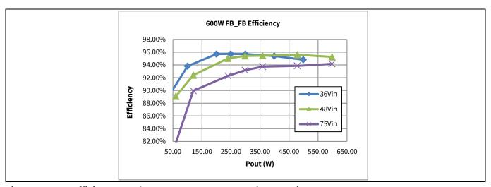
Figure 14 Efficiency results at 36 V DC, 48 V DC, and 75 V DC input
