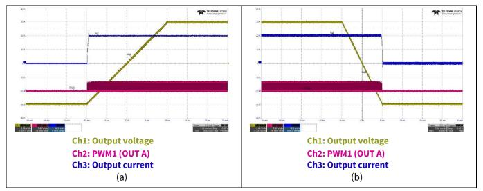
Figure 24 Evaluation kit soft start and soft stop waveforms at 20 A load - a) TON\_RISE = 20 ms, b)
