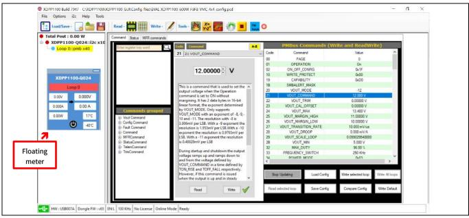
Figure 12 GUI with connected XDPP1100-Q024 and the loaded design file
