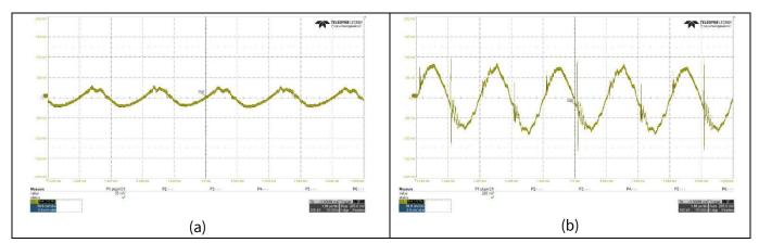
Figure 15 Output voltage ripple (AC coupled mode) - a)  $V_{IN} = 48 \text{ V}$ ,  $I_{OUT} = 0 \text{ A}$ , b)  $V_{IN} = 72 \text{ V}$ ,  $I_{OUT} = 50 \text{ A}$
