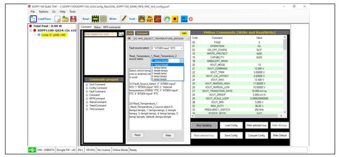
Figure 44 Configure temperature sensors through the PMBus command MFR\_SELECT\_TEMPERATURE\_SENSOR (Code DC)
