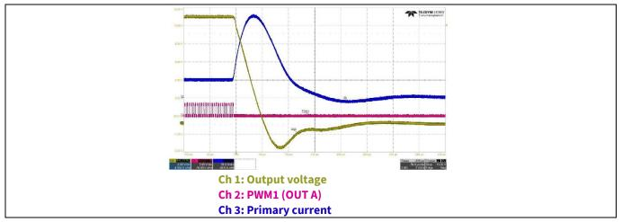
Figure 40 **Short-circuit protection**
