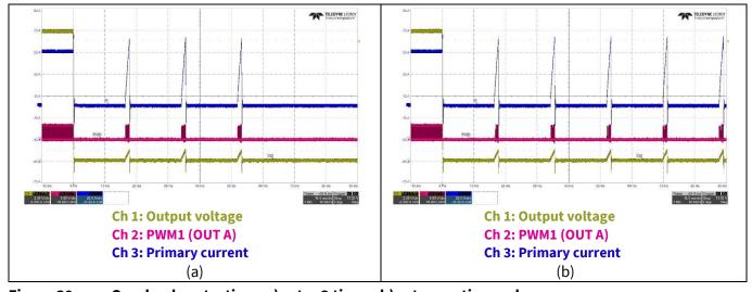
Figure 39 Overload protection - a) retry 3 times, b) retry continuously
