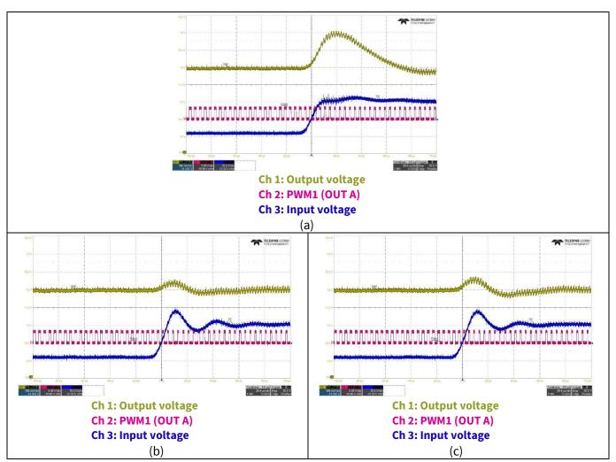
Figure 50 Feed-forward experimental results - a) feed-forward disabled by selecting pid0\_ff\_override\_sel as pid0\_ff\_override and pid0\_ff\_override = 0, b) same cycle enabled, c) same cycle disabled
