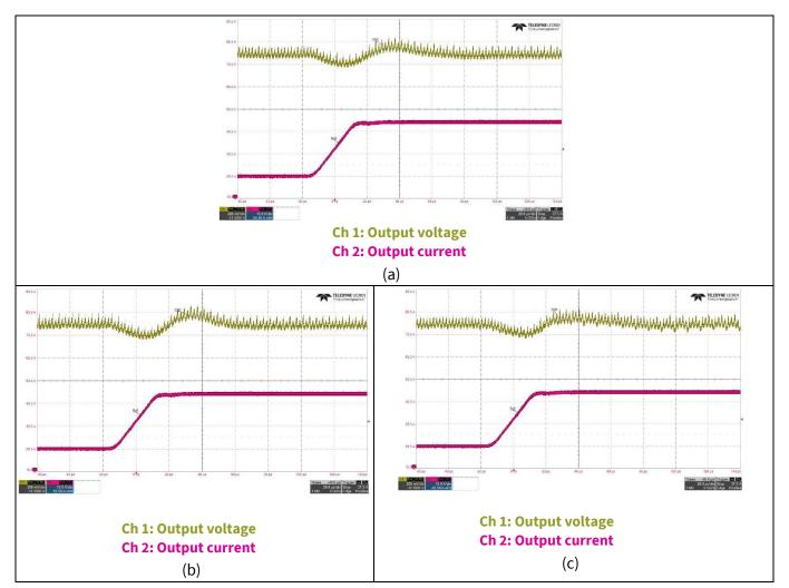
Figure 54 Flux balancing load transient results - a) ramp0\_dutyc\_lock = unchecked (flux balancing disabled), b) ramp0\_dutyc\_lock = checked and fbal\_time\_only = enable (flux balancing is disabled due to DCM), c) ramp0\_dutyc\_lock = checked and fbal\_time\_only = disable (flux balancing enabled with volt × seconds technique)
