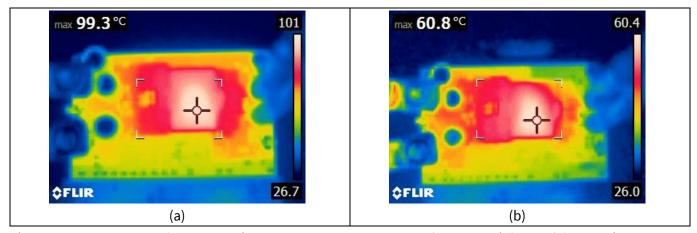
Figure 5 Thermal performance with  $V_{IN}$  = 48 V and  $I_{OUT}$  = 25 A - a) natural airflow, b) fan cooling
