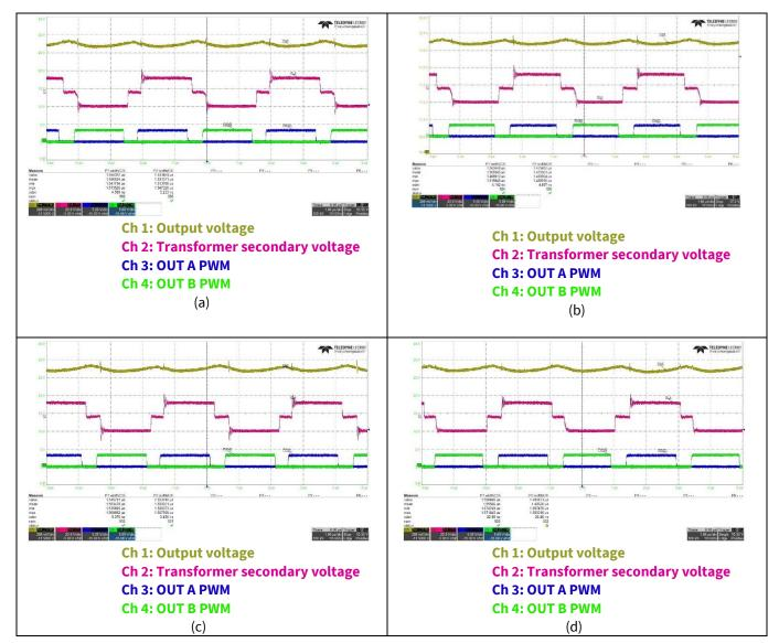
Figure 52 Flux balancing steady-state result - a) ramp0\_dutyc\_lock = unchecked (flux balancing disabled), b) ramp0\_dutyc\_lock = checked and Iout = 10 A (flux balancing is disabled due to DCM), c) ramp0\_dutyc\_lock = checked and fbal\_time\_only = enable (flux balancing is disabled due to DCM), d) ramp0\_dutyc\_lock = checked and fbal\_time\_only = disable (flux balancing enabled with volt × seconds technique)
