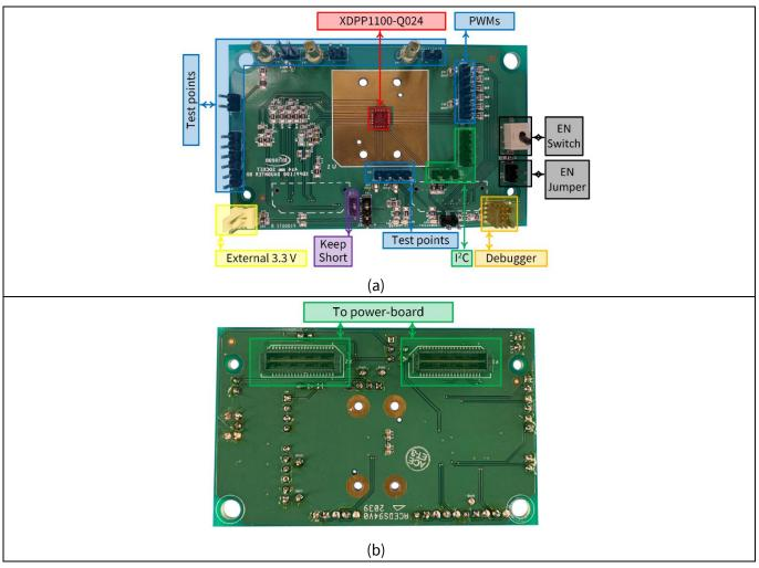
Figure 3 Daughterboard - a) top view, b) bottom view
