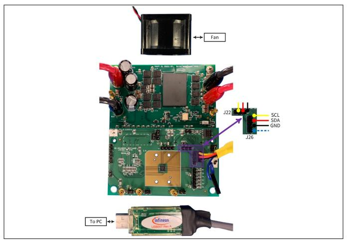
Figure 4 **Evaluation test set-up**
