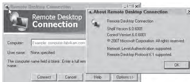
FIGURE 7.2 Verifying NLA support in RDC
