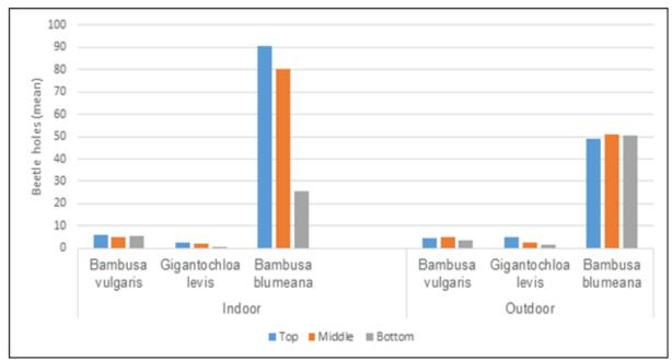
**Fig. 3.** Mean number of beetle holes per section per bamboo species exposed to indoor and outdoor environment after 13 weeks of feeding test.
