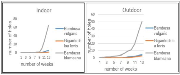
Fig. 2. Cumulative number of beetle holes after 13 weeks of feeding test.
