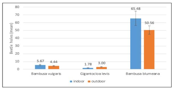
**Fig. 4.** Mean number of beetle holes as affected by the indoor and outdoor setting after 13 weeks of feeding test (mean  $\pm$  SEM).
