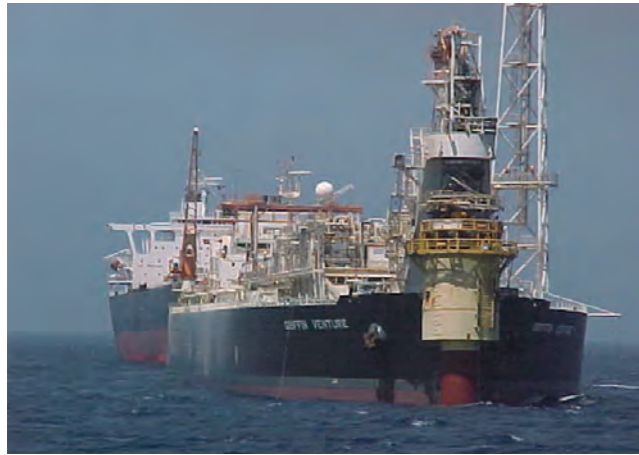
GRIFFIN VENTURE , the FPSO vessel used for offshore processing and storage of oil from the Griffin oil fields
