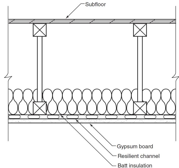
FIGURE A.8.15.1.2.6 Combustibile Concealed Space Cross Section.
