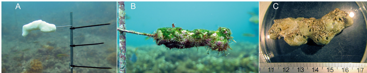
Fig. 2. Experimental setting showing (A) a freshly deployed coral cylinder, (B) a cylinder after about 7 mo underwater, and (C) a retrieved cylinder with fouling removed (borer holes — here from bivalves — are easily seen)
