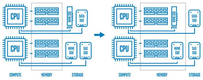
Figure 2: Intel<sup>®</sup> Memory Drive Technology modifies a part of the system's storage to transparently serve as system memory.
