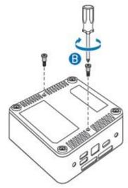
2. Attach the two slightly larger black screws to the bottom chassis cover of the Intel NUC.
