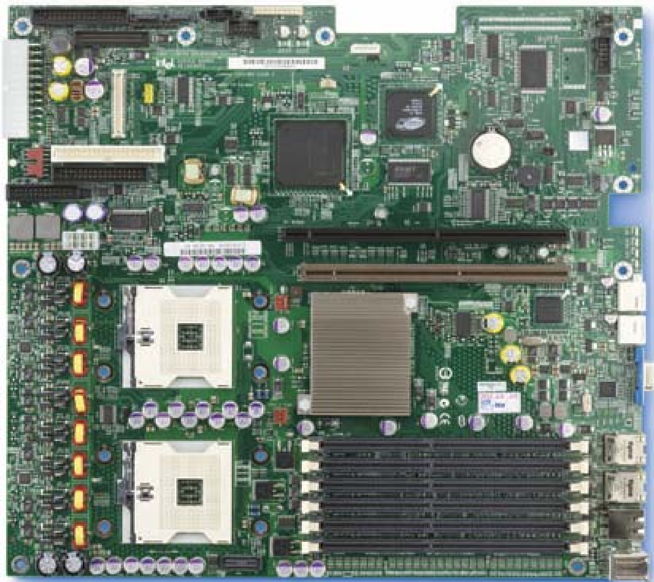
Figure 41. Intel® Server Board SE7320VP2 Board Layout
