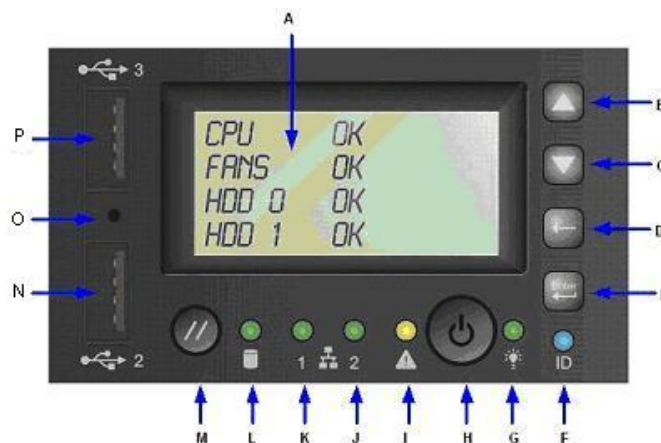
Figure 35. Intel Local Control Panel Overview
