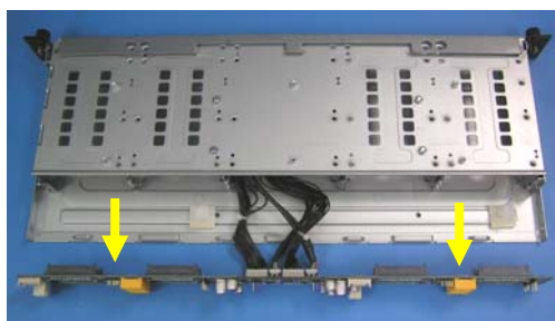
Figure 52. Front Panel Cables
