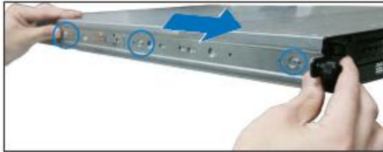
Figure 37. Attaching the Front End of the Server Rail to Side of Chassis
