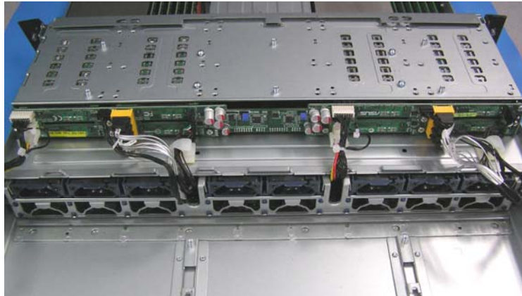
Figure 53. Cable Bundles in the Hard Disk Drive Bay Module
