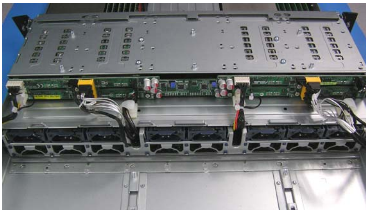
Figure 51. Connected Cables and Backplane Expose
