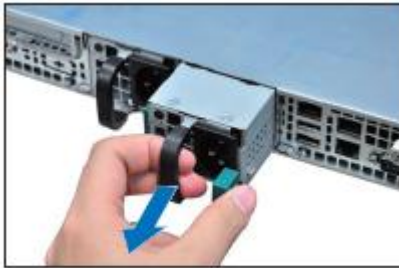
Figure 43. Pulling Out the Failed PSU
