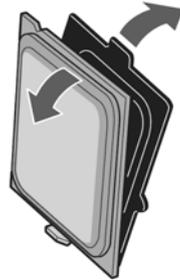
**Figure 16. Remove Processor Protective Cover**
