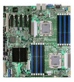
Figure 1. Intel<sup>®</sup> Server Board S5520HC/S5520HCT
