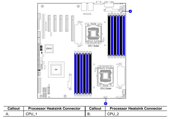
Figure 20. Locating Active Heatsink Cable Connections
