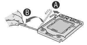
Figure 13. Opening the Processor Socket Lever
