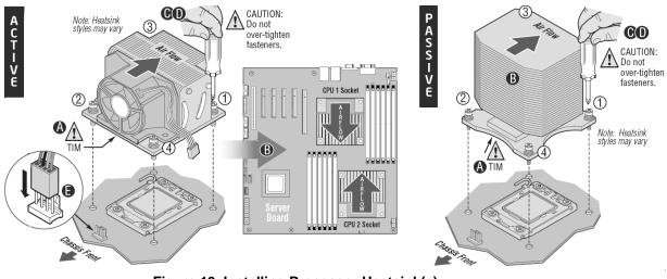
Figure 19. Installing Processor Heatsink(s)
