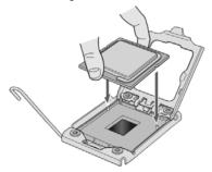
Figure 17. Install the processor
