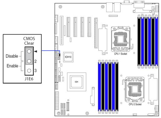
Figure 11. CMOS Clear Jumper
