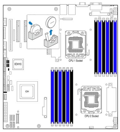
Figure 21. Locating and Removing the CMOS Battery
