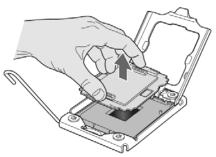
Figure 15. Removing the Processor Socket Protective Cover
