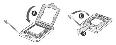
Figure 18. Close Load Plate and Socket Lever
