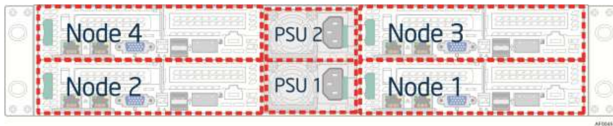
Figure 2. Compute Node Scheme (Rear View)
