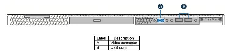
Figure 30. Front I/O Panel Features
