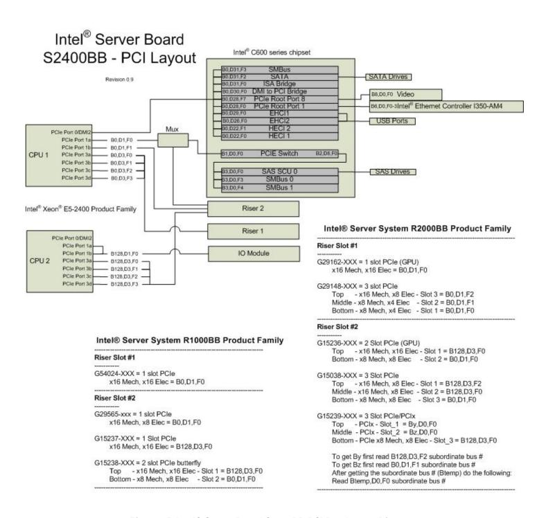
Figure 35. Intel® Server Board S2400BB PCI Bus Layout Diagram
