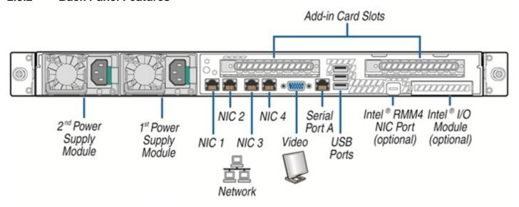
Figure 5. Back Panel Feature Identification
