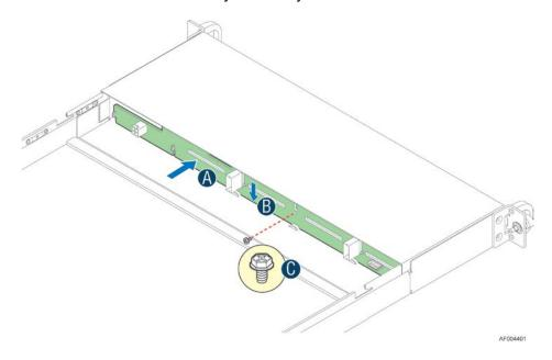
On the front side of each backplane are mounted eight hard disk drive interface connectors (A), each providing both power and I/O signals to attached hard disk drives.
