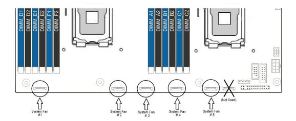
Figure 22. Server Board System Fan Connector Locations
