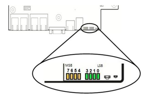
Figure 42. POST Diagnostic LEDs
