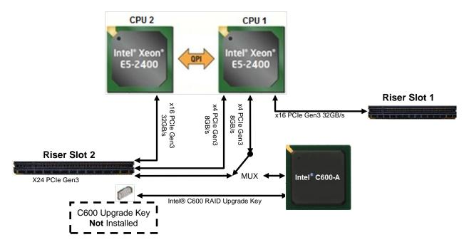
Figure 33. Riser Slot Architecture - Intel® C600 Upgrade Key NOT installed
