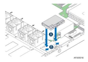
Figure 29. AXXBBU09 and AXXRFMBU2 Installation
