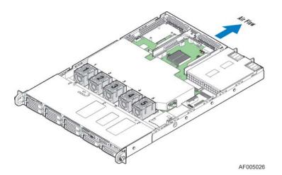
Figure 21. System Fan Identification
