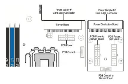
Figure 17. Main Power Connector Identification
