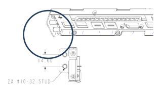
Figure 19. Chassis Grounding Studs
