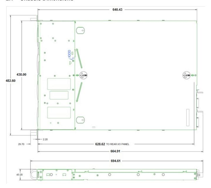
Figure 1. Chassis Dimensions
