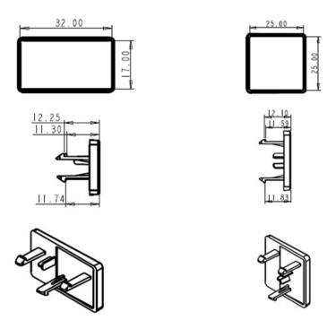
Figure 13. Front Bezel accessory ID Badge mechanical drawings
