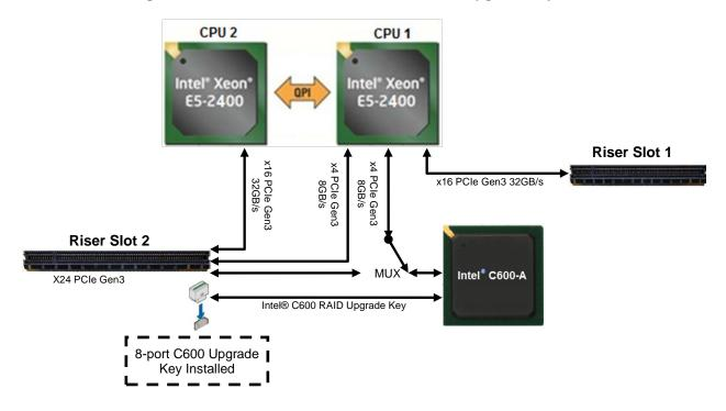
Figure 34. Riser Slot Architecture - Intel® C600 Upgrade Key Installed
