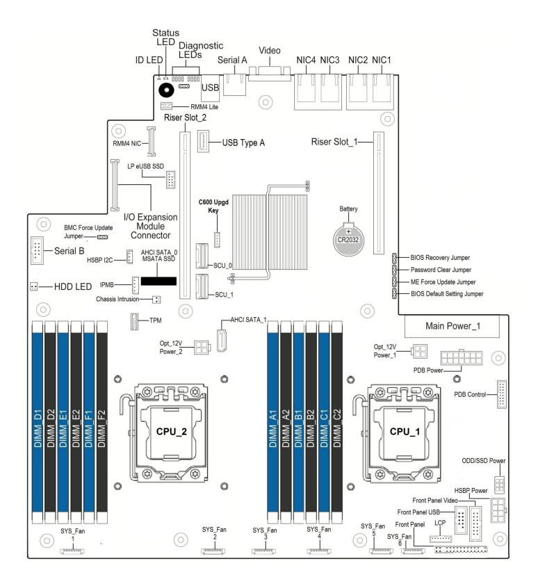
Figure 7. Intel<sup>®</sup> Server Board S2400BB
