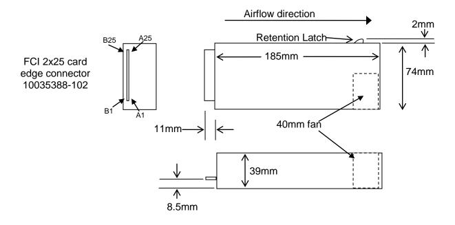
Figure 14. Power Supply Module Mechanical Drawing
