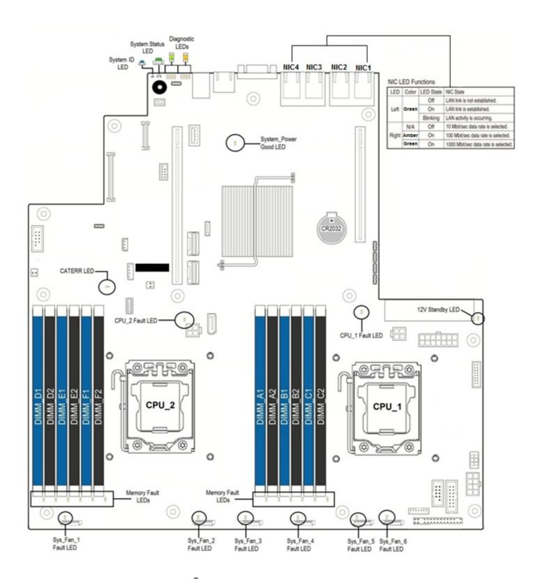
Figure 8. Intel<sup>®</sup> Light-Guided Diagnostic LEDs - Server Board
