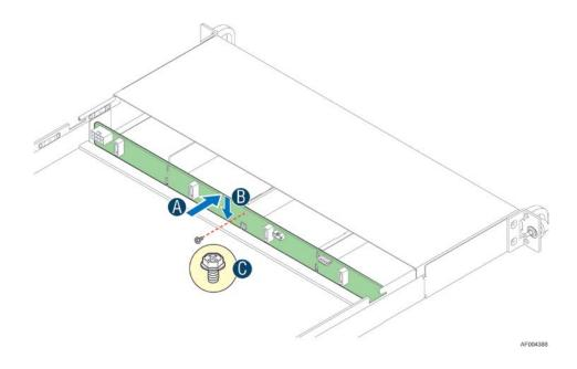
On the front side of each back plane are mounted four hard disk drive interface connectors (A), each providing both power and I/O signals to attached hard disk drives.
