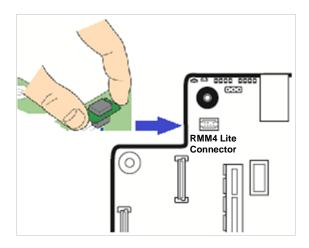
Figure 40. Intel® RMM4 Lite Activation Key Installation
