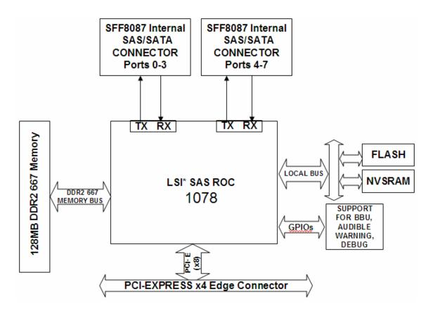
Figure 1. Hardware Block Diagram
