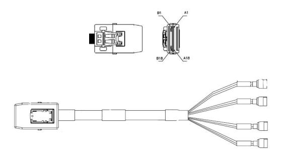
Figure 5. SFF8087 to Four-port Internal Cable
