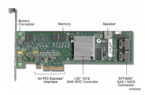
Figure 2. Intel® RAID Controller SRCSATAWB Physical Layout
