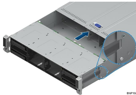
Figure 47. Installing the chassis drive cage – insert drive cage
