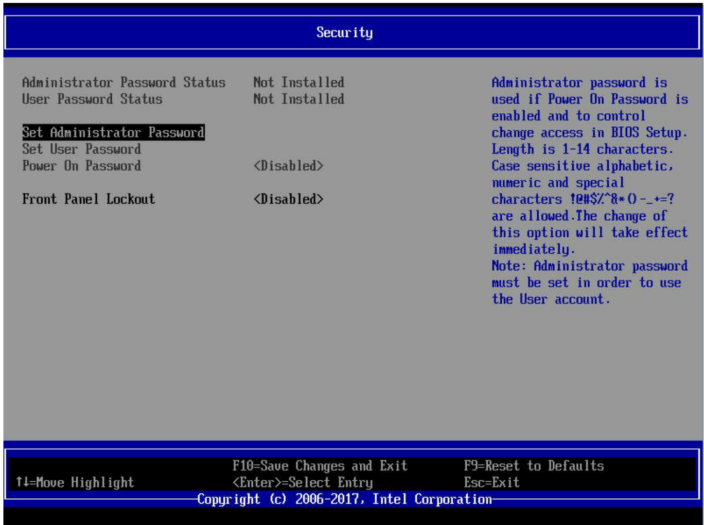
Figure 110. Security Tab of BIOS Setup Utility
