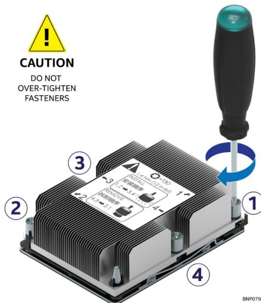
Figure 17. Installing the PHM
