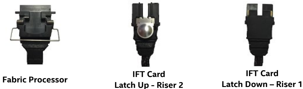
Figure 76. Internal Fabric Cable Connector Identification
