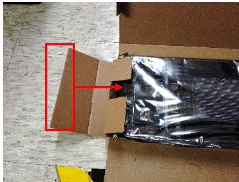
Figure 125. Compute Module Packaging Assembly Instructions - 4
