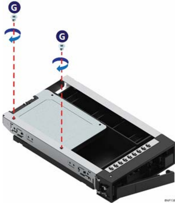
Figure 43. 3.5" Drive carrier to 2.5" SSD bracket – secure SSD to carrier
