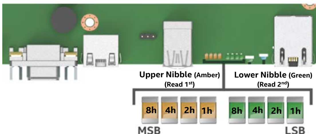
Figure 97. POST diagnostic LED location
