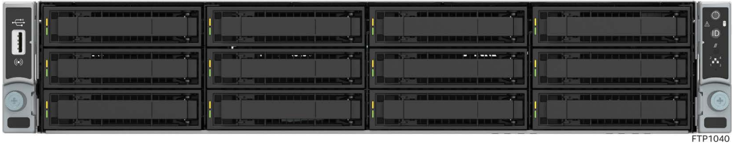
Figure 76. 12 x 3.5" Drive bay configuration (Intel® Server System R2312WFTFxxx – storage system)
