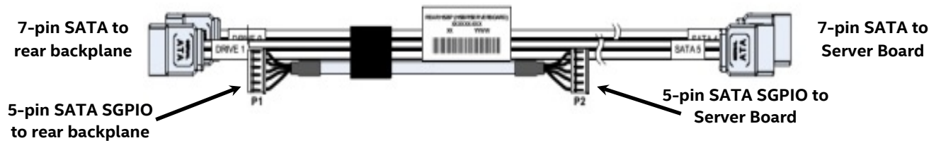
Figure 70. Rear HSBP SATA & SGPIO cable bundle
