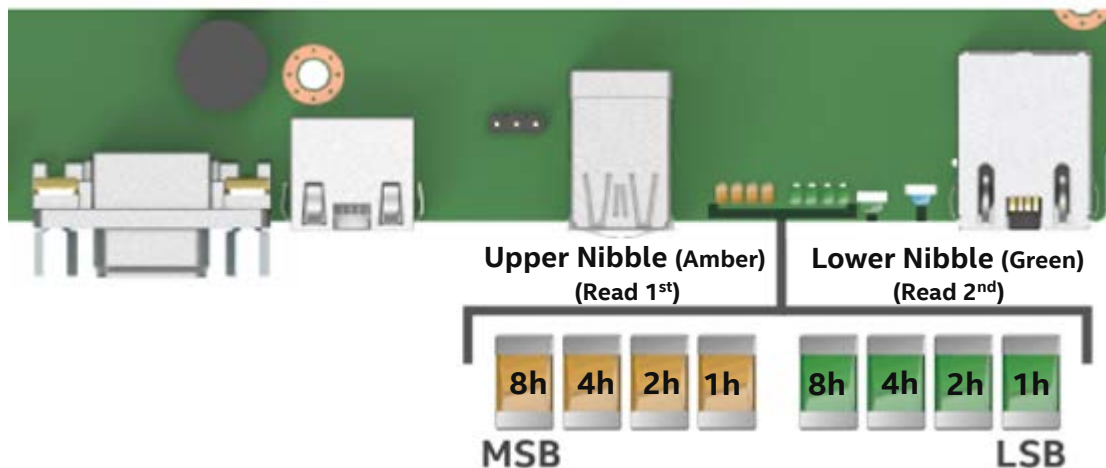
Figure 87. Onboard POST diagnostic LEDs
