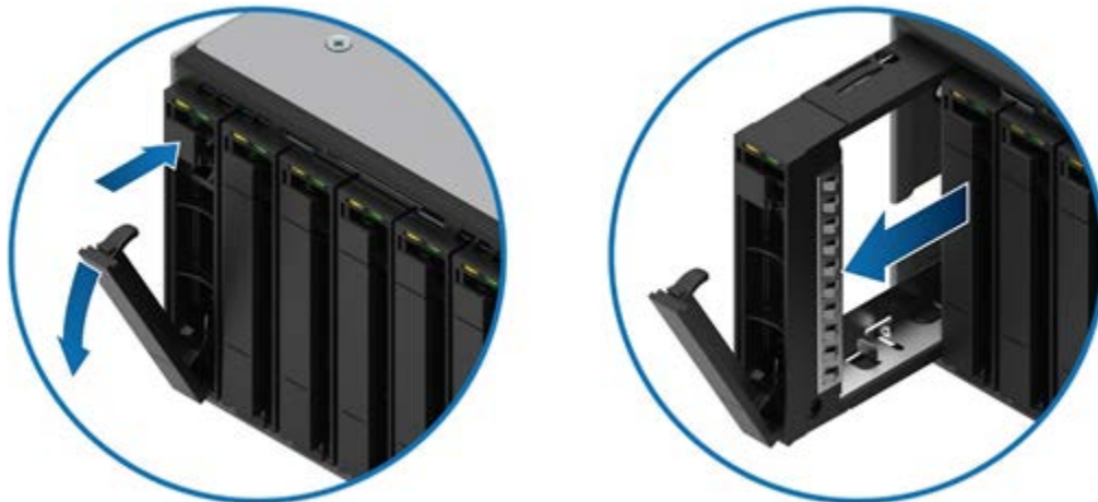
Figure 38. Drive carrier removal
