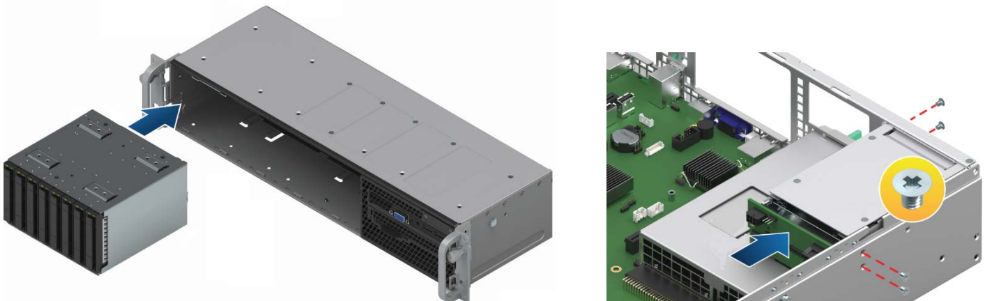
Figure 43. 2.5” drive bay module placement options
