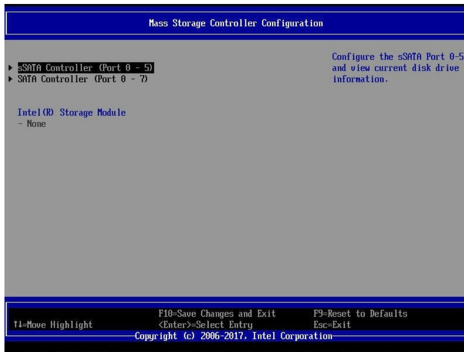
Figure 55. BIOS setup Mass Storage Controller Configuration screen
