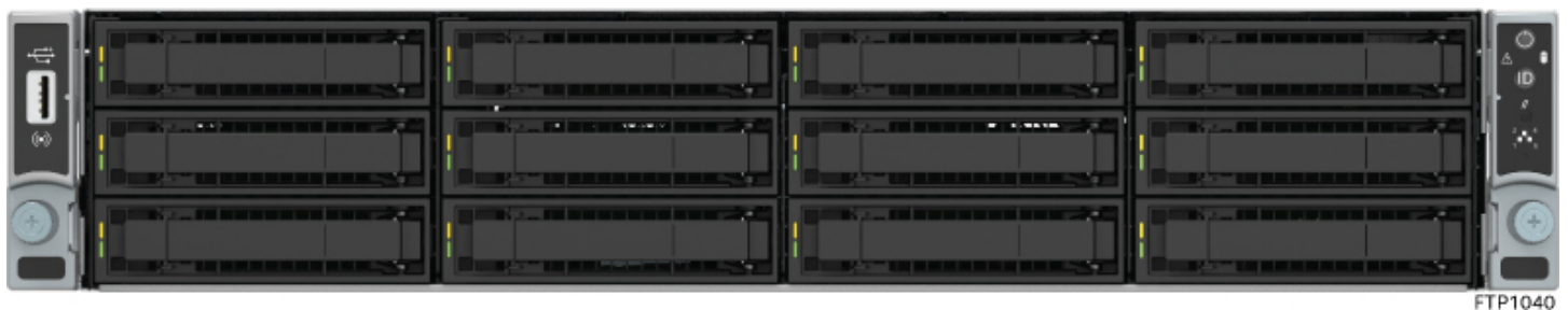
Figure 10. 3.5" x 12 front drive bay configuration – LFRB2312WFTFxxx
