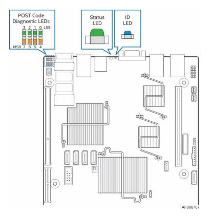
Figure 53. Diagnostic LED Placement Diagram
