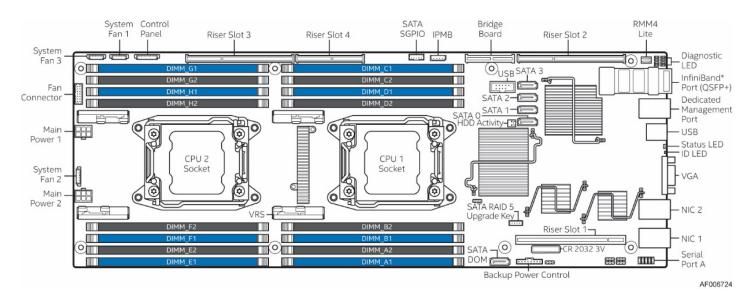
Figure 3. Server Board Components (S2600TPFR)
