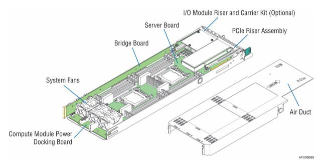
Figure 4. Compute Module Components
