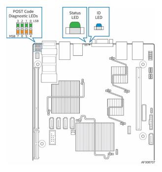
Figure 48. Rear Panel Diagnostic LEDs
