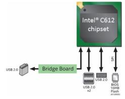
Figure 43. USB Ports Block Diagram
