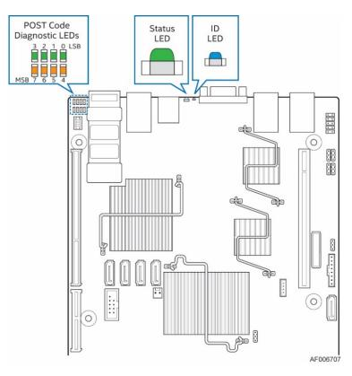
Figure 8. Intel<sup>•</sup> Light Guided Diagnostic LED
