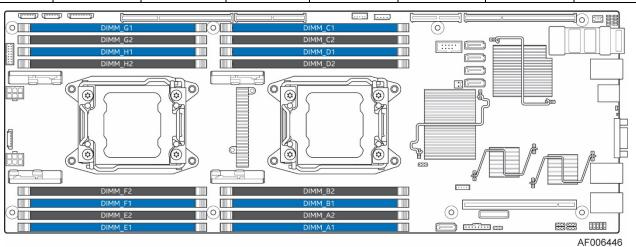
Figure 36. Intel<sup>®</sup> Server Board S2600TPR Product Family DIMM Slot Layout
