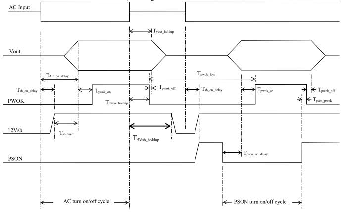
Figure 51. Turn On/Off Timing (Power Supply Signals – 5VSB)
