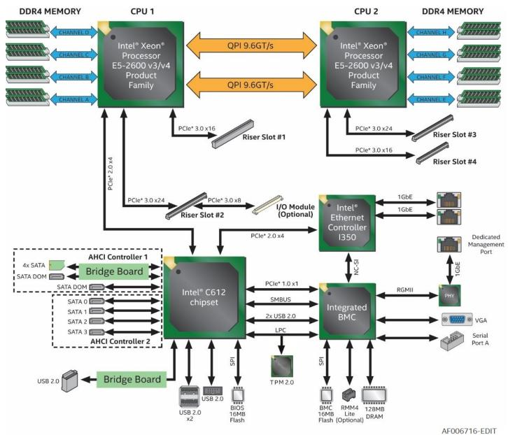
Figure 14. Intel<sup>®</sup> Server Board S2600TPTR Block Diagram
