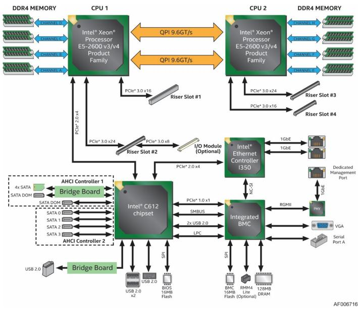
Figure 12. Intel<sup>®</sup> Server Board S2600TPR Block Diagram
