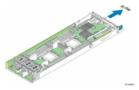
Figure 50. Air Flow and Fan Identification
