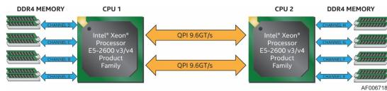
Figure 35. Integrated Memory Controller Functional Block Diagram
