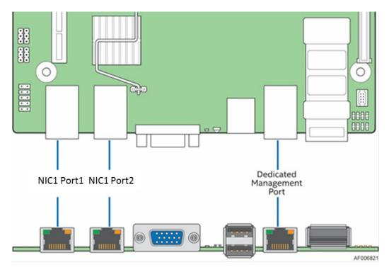
Figure 41. Network Interface Connectors
