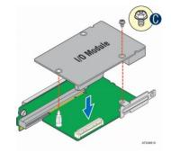
Figure 22. I/O Module Carrier Installation
