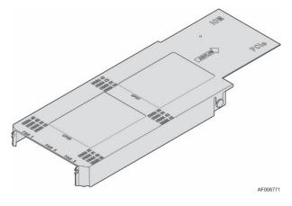
Figure 27. Air Duct
