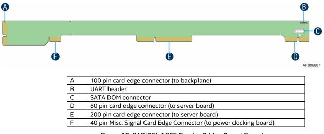
Figure 19. SAS/PCIe\* SFF Combo Bridge Board Overview
