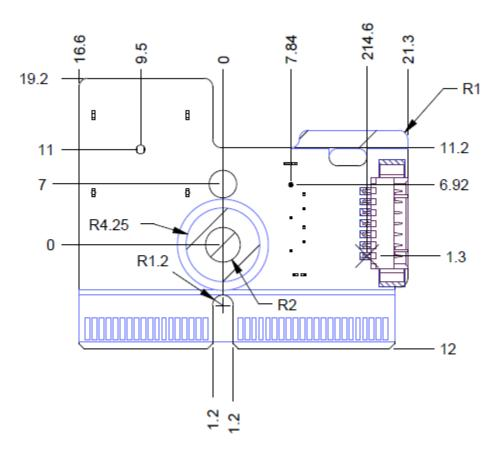
Figure 31. Breakout Board Mechanical Drawing (Unit: mm)
