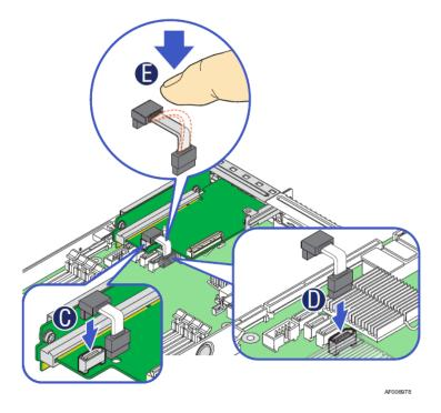
Figure 25. Connecting the M.2 SATA Cable
