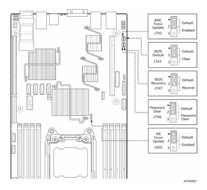
Figure 9. Jumper Identification
