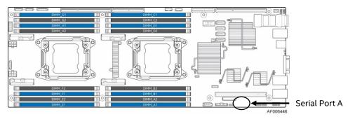
Figure 44. Serial Port A Location
