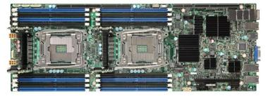
Figure 1. Intel<sup>®</sup> Server Board S2600TPFR (demo picture)
