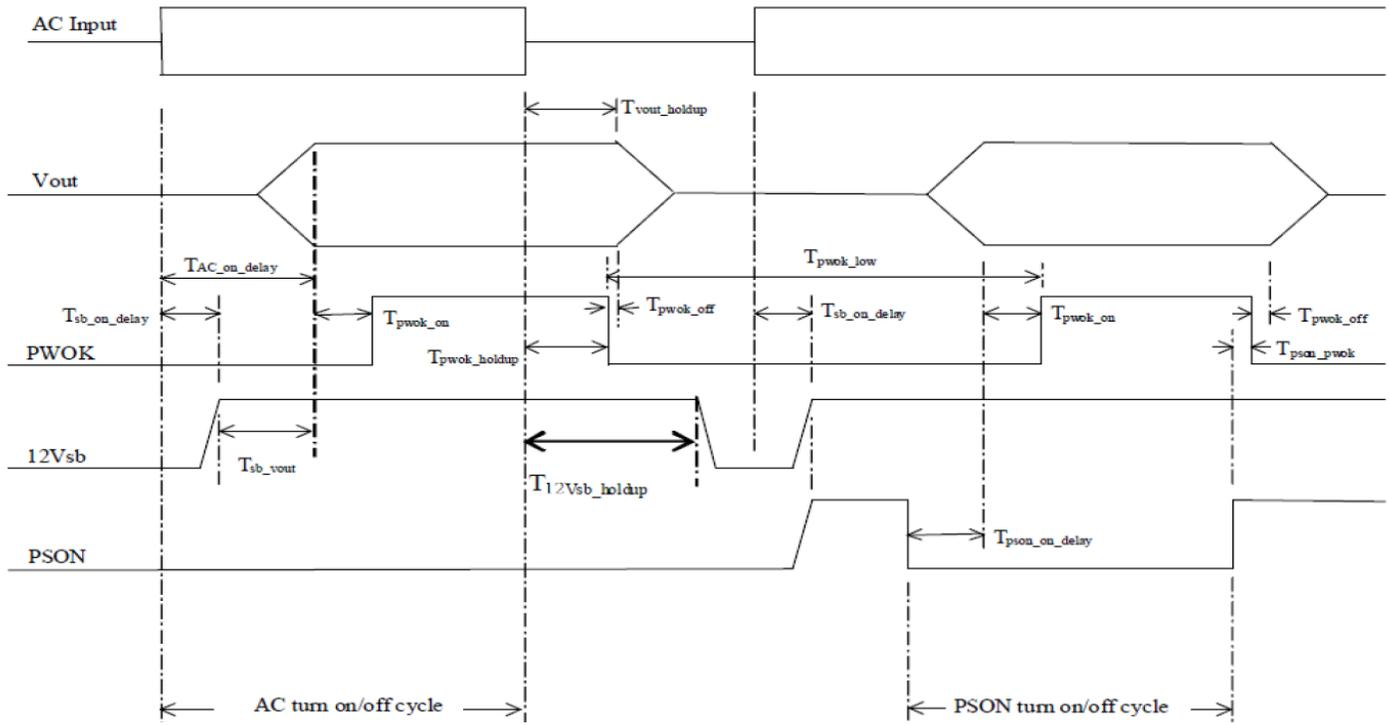
Figure 52. Turn On/Off Timing (Power Supply Signals – 12VSB)
