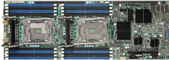
Figure 1. Intel® Server Board S2600TPFR (demo picture)
