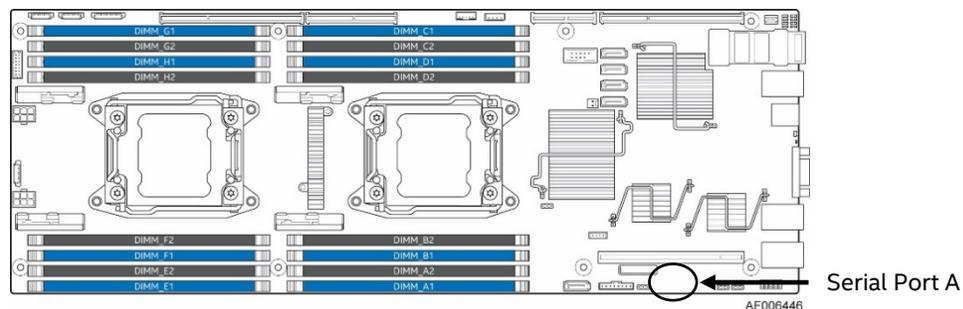
Figure 44. Serial Port A Location
