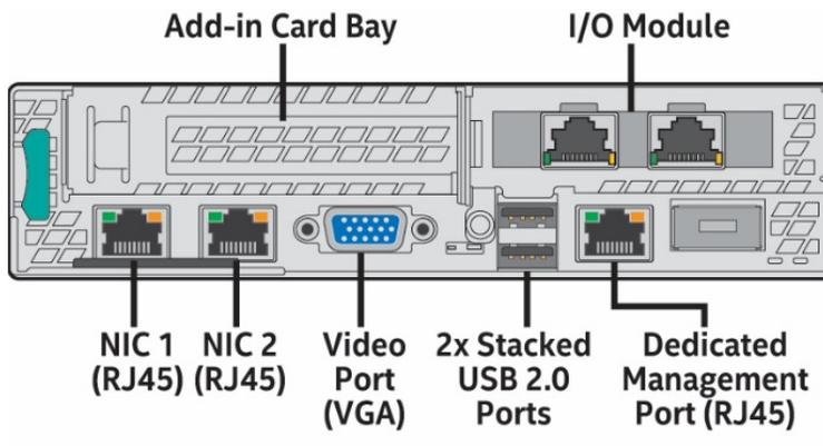
Figure 7. HNS2600TP24R Compute Module Back Panel
