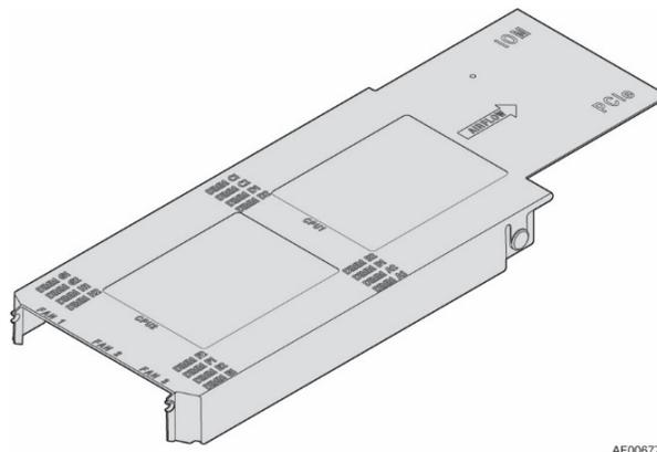
Figure 27. Air Duct
