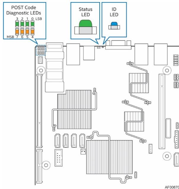
Figure 48. Rear Panel Diagnostic LEDs
