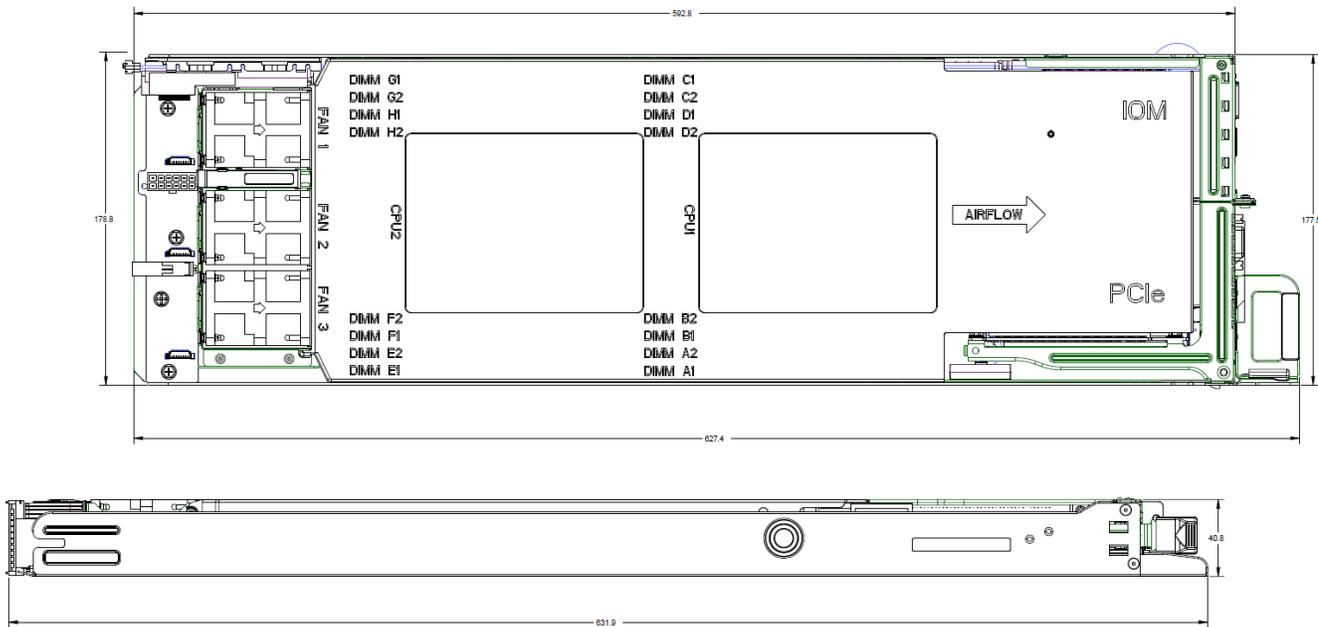
Figure 11. Compute Module Dimension
