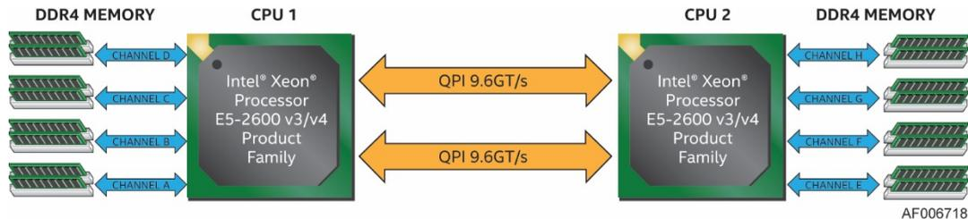
Figure 35. Integrated Memory Controller Functional Block Diagram
