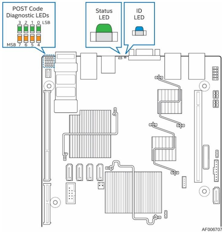
Figure 8. Intel® Light Guided Diagnostic LED
