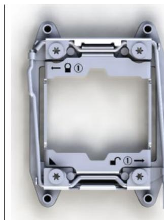
Figure 33. Processor Socket ILM
