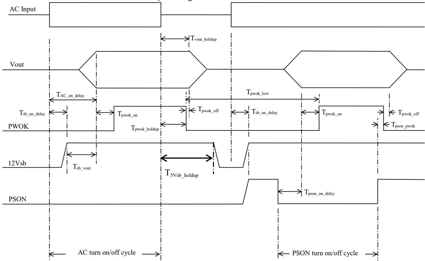
Figure 51. Turn On/Off Timing (Power Supply Signals – 5VSB)
