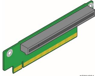
Figure 20. Riser Card for Riser Slot #1
