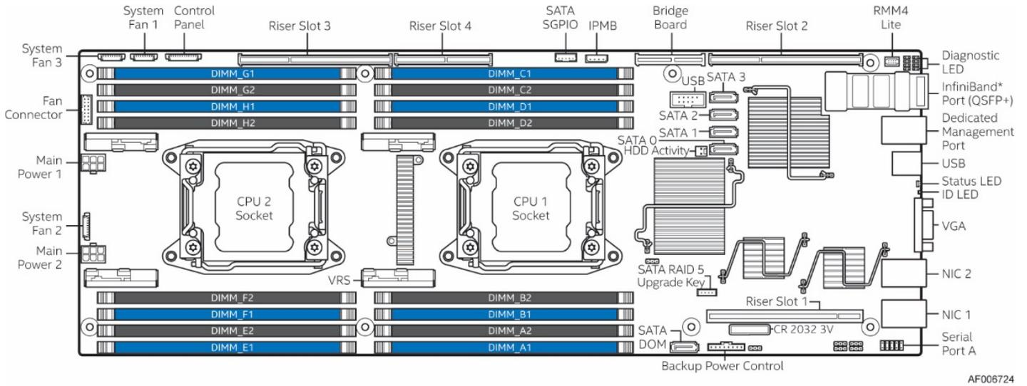
Figure 3. Server Board Components (S2600TPFR)
