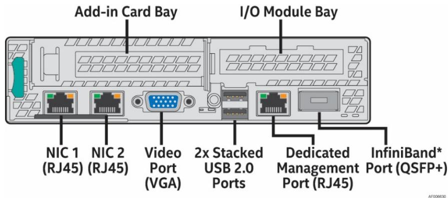
Figure 6. HNS2600TPR Compute Module Back Panel
