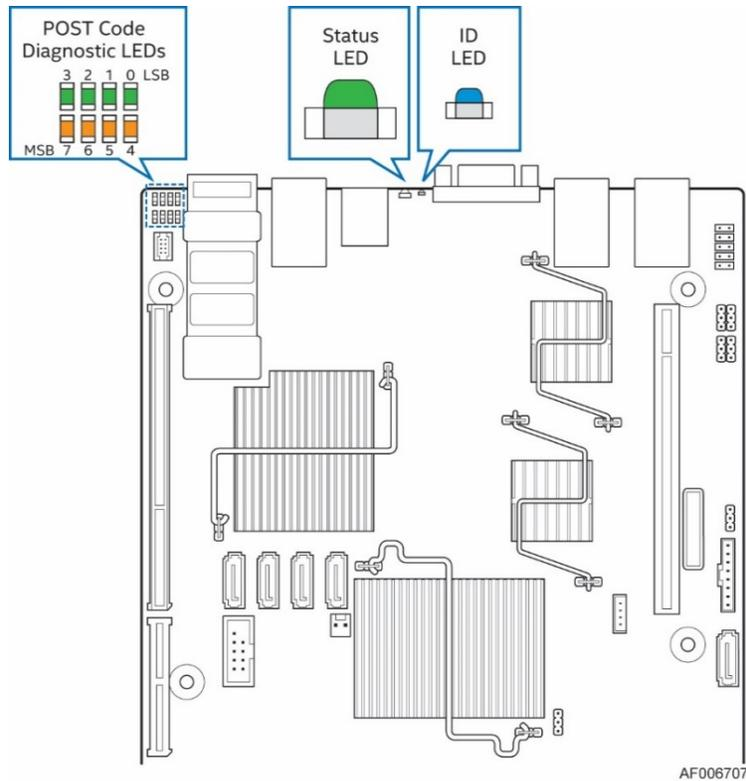
Figure 53. Diagnostic LED Placement Diagram
