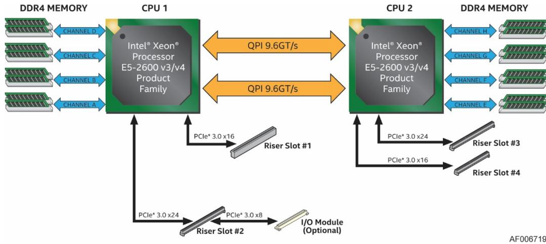
Figure 37. Add-in Card Support Block Diagram (S2600TPR)
